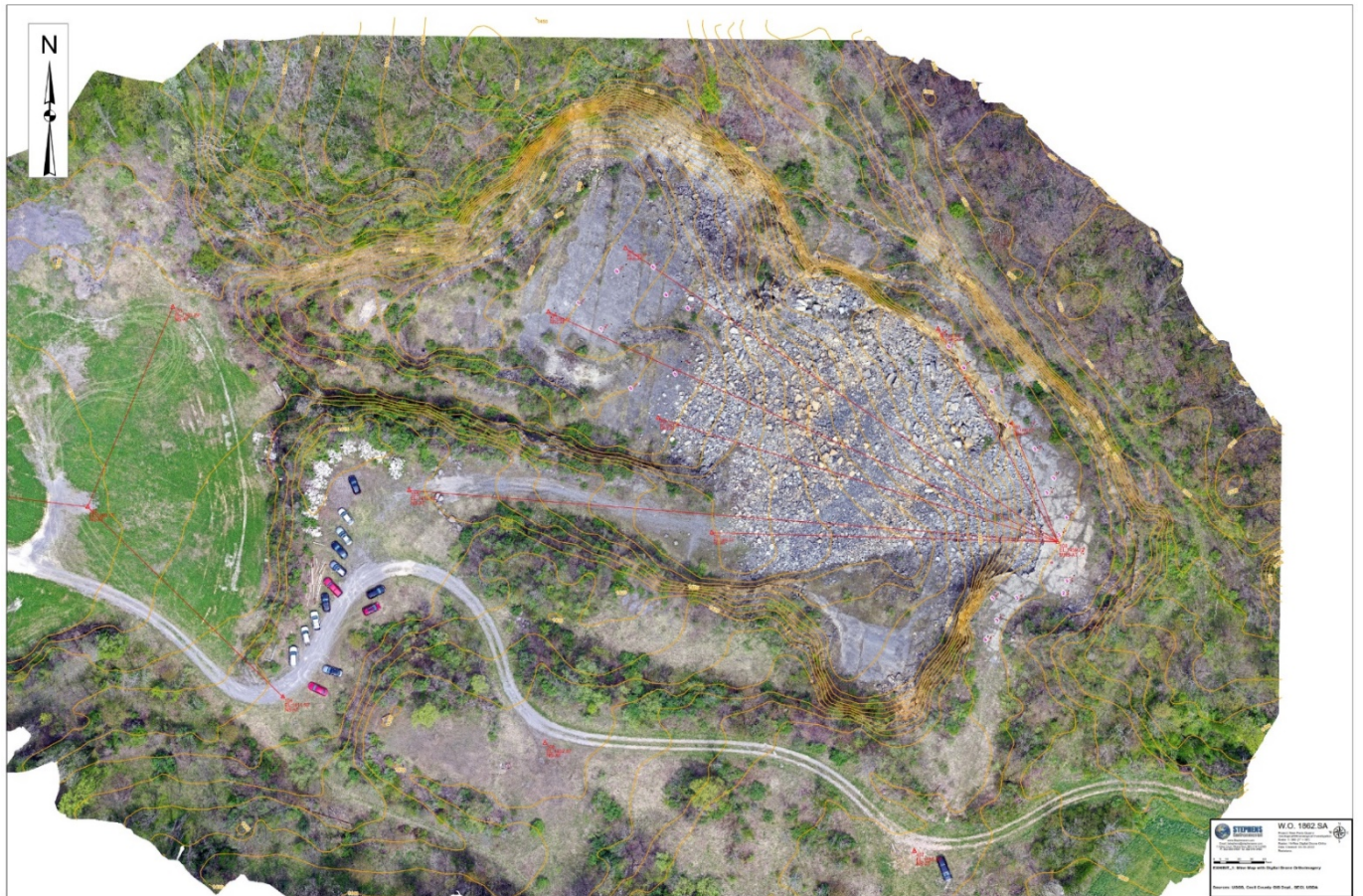
Hi Resolution Digital Ortho mosaic prepared from over 700 individual nadir camera shots taken as a mapping mission using a Mavic 2 Pro drone. The cameras were processed in DroneDeploy with a dozen survey quality ground control points. 5 Feet contours exported from Drone Deploy show current topography at the quarry on the flight date 04-30-2022. The red lines indicate intervisibility between Network GPS and conventionally surveyed GCPs.
