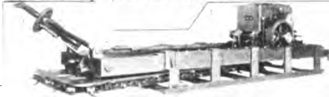
2 Jeffrey Mfg Co Chain Coal Cutter Side View.
