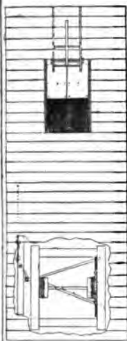
Plan of Top of Tipple Showing Scales Connection.
