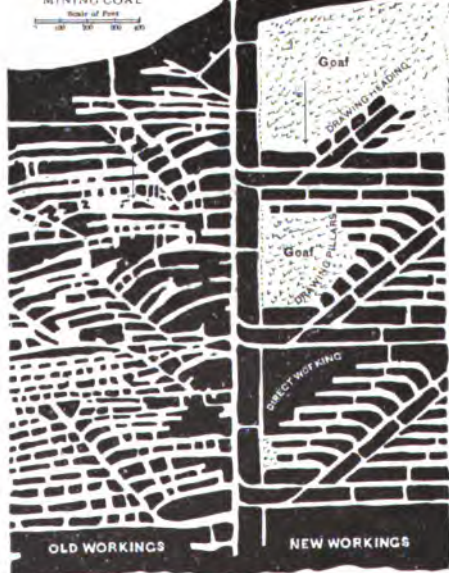
Fig. 3. PLAN ILLUSTRATING OLD and NEW METHODS OF MINING COAL
